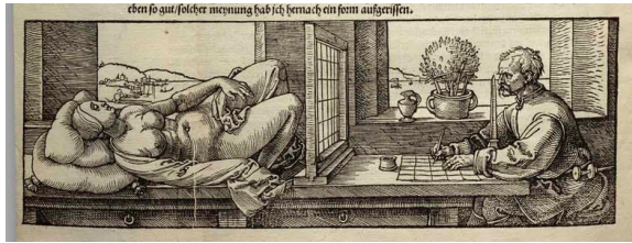
Figure 10: De Symmetria and Underweysung der Messung, Albrecht Dürer (1532). An alternative perspective machine, the rectangular frame and adjustable eyepiece are the same as Figure 8, however, instead of drawing directly on a sheet of glass placed in the frame, a square grid is strung in the frame and duplicated on the paper where the final picture is drawn.
